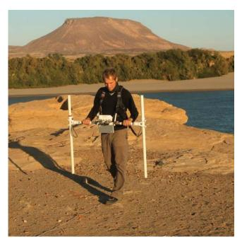
cassette and either one or two Grad-01-1000L sensors mounted on a rigid carrying bar— is now complemented by the addition of a Non-Magnetic Cart, which enables Grad601 equipment to be mounted on a multi-sensor platform. Combined with the logging software and GPS, this lets existing Grad601users either upgrade to a multi-acquisition platform or use the standard handheld version, depending on field constraints.
