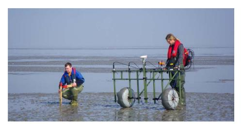
Fig. 3 Magneto MXPDA 5-channel cart system during a survey session at the Wadden Sea with customized wheels
