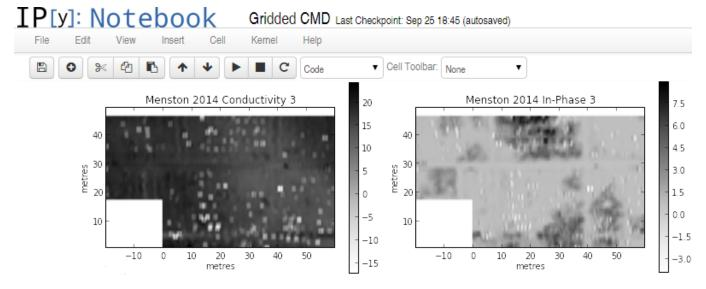
Fig. 1 Automated management and re-gridding of electromagnetic induction data, allowing an easy, streamlined importation into conventional data processing packages.
