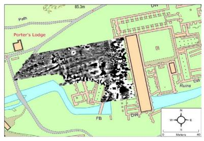
Fig. 3 CartEasyN system at 0.25 m x 0.25 m with Bartington 1000L fluxgate sensors.
