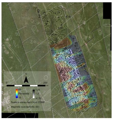
Fig. 2 YDMP transcriptions, magnetic susceptibility survey, EMI survey and magnetic survey, north of High Pasture, Grassington (aerial imagery (c) Google 2014).
