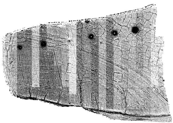
Fig. 1 Raw Bartington Grad-601 datasets indicating typical systematic errors.
