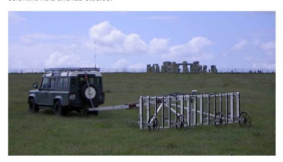
Fig. 4 Magneto MX 16-channel system during a survey session at Stonehenge
