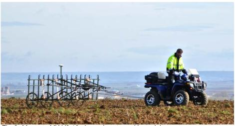
Fig. 2 Magneto MX V3 16-channel system with modular cart
