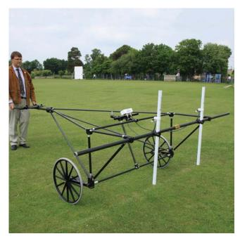
Up to 12 Grad-13 or Grad601sensors can be mounted on the lightweight Non-Magnetic Cart, enabling a far wider and quicker coverage of the area being surveyed. The 4 metre, 20kg cart is constructed from a set of carbon fibre tubes with a single tool used to operate all locks and catches. It can be pushed or towed by a single operator, or be configured for towing behind a small vehicle with an additional 4 metre, 9kg attachment.
