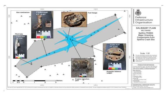
Fig. 2 Map of the Spitfire P95903 aircraft parts excavation
