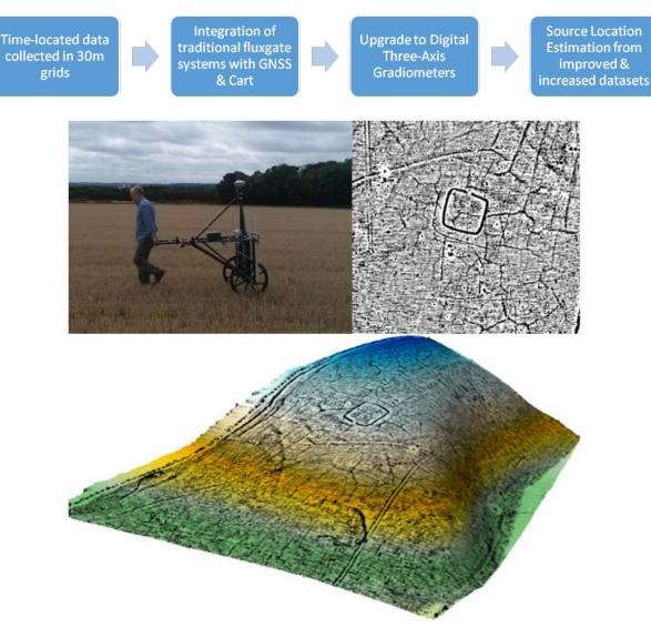
Fig. 2 Clockwise: CartEasyN collection system, Minimally processed greyscale of CartEasyN data, CartEasyN data overlaying topographic model
