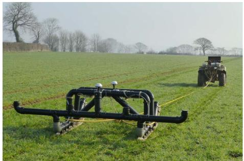
Fig. 1 Sledge systems such as ArchaeoPhysica's 'Blackbird' can achieve over 20ha of Cs magnetometer and EMI survey coverage a day, at greater resolution and data quality than walked survey
