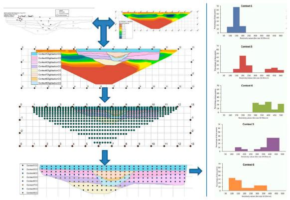
Fig. 1 Extraction of resistivity data from ERI profiles into separate archaeological contexts
