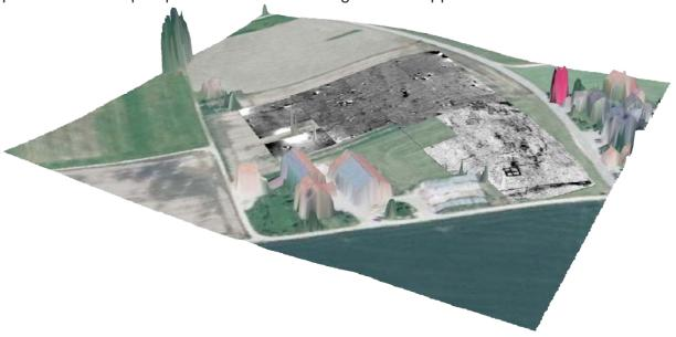
Fig. 1 Weildorf. Cäsium-Magnetometer Smartmag SM4G-Special, Duo-Sensor-configuration. sensitivity +-10pT, 0,50 m x 0,25 m sampling interval, interpolated to 0,125 x 0,125 m, 40-m-grid. Radargram depth slice 40 - 60 cm, GSSI SIR-3000 with 400 MHz-antenna, prospected area 109 x 80 m. sampling interval 2 x 25 cm (BLfD, Archiv-Nr. 8142/073\_1).
