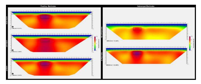
Fig. 2 Inversion results between protocols (a) dipole-dipole, (b) pole-dipole and (c) gradient, using floating electrodes (left side) and using submerged electrodes position with (d) or without (e) a priori information (right side). Black dots indicate electrode position.
