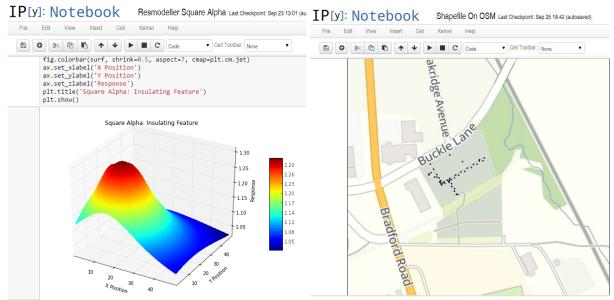
Fig. 2 Numerical modelling and display of resistivity responses over three-dimensional features.
