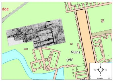
Fig. 2 MALÅ Mira Mini 1.83 m depth slice results, referenced with a robotic total station.
