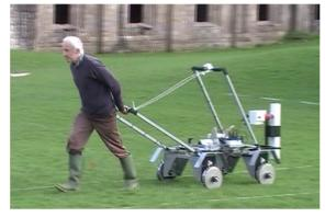
Research ADVANCED RM85 Resistance Meter and Expansion Port Interface Box 1 are mounted centrally. Provision is made for attaching a towing system.
