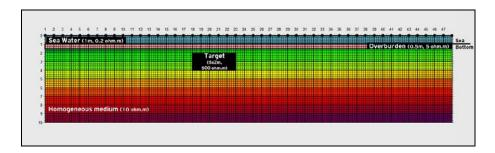
Fig. 1 Synthetic model for ERT marine for shallow sea water measurements. A target (500 ohm.m) is embedded in a homogeneous medium (10 ohm.m), 0.5m below an overburden layer (5 ohm.m). Sea water column is set to 0.5 m (resistivity 0.2 ohm.m).
